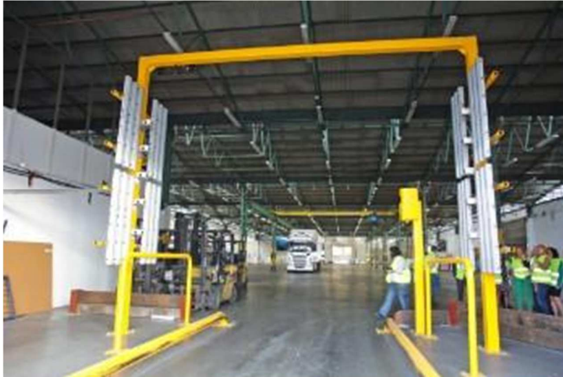
Figure 34: Picture of the Palletways Archway Scanning System
