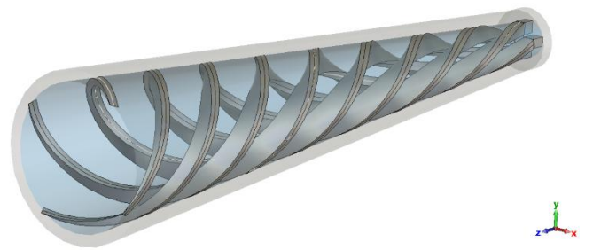
Fig. 1. 3D view of the proposed conical horn antenna with emphasised intertwined exponential ridges
