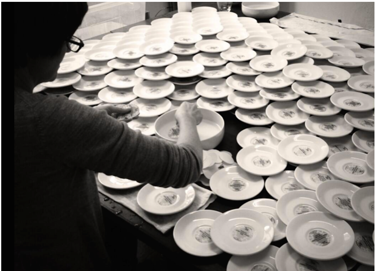
Opposite: The industrial firings of the cups and saucers for the exhibition. Above: The decal transfers being applied by hand to each of the 1550 cups and saucers.
