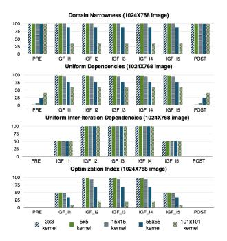
Fig. 9. Domain narrowness, uniform (inter-iteration) dependencies and optimization index estimation for the IGF on different kernel sizes
