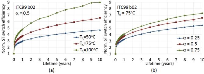
Fig. 5. Profile of the normalized ST switch efficiency over time for *b02* benchmark (normalization factor:  $SwEDC_0(b02) = 1.02 \times 10^7$ ) with: (a) different aging temperatures; (b) different stress ratios.
