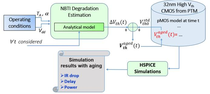
Fig. 2. Simulation flow with embedded aging effects.
