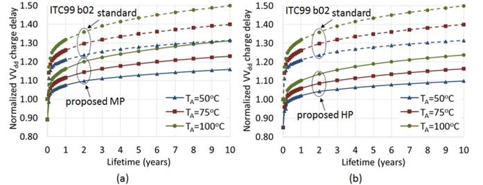
Fig. 9. Profile over time of the normalized  $VV_{dd}$  charge delay during the wake-up protocol for the *b02* benchmark (normalization factor:  $\tau_{VVdd0}(b02) = 32.4ps$ ) with: (a) MP ST design; (b) HP ST design.
