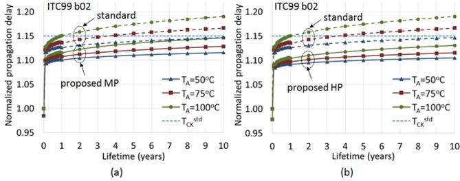
Fig. 8. Profile over time of the normalized propagation delay for the *b02* benchmark (normalization factor:  $\tau_{wc0}(b02) = 52.8ps$ ) with: (a) MP ST design; (b) HP ST design.
