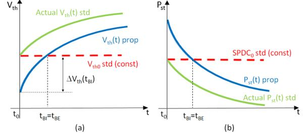
Fig. 6. Schematic representation of the proposed method to determine ST  $V_{th}$  optimal value: (a) qualitative  $V_{th}$  trend over time for the proposed (prop) and standard (std) ST design, and (b) correspondent static power trend.
