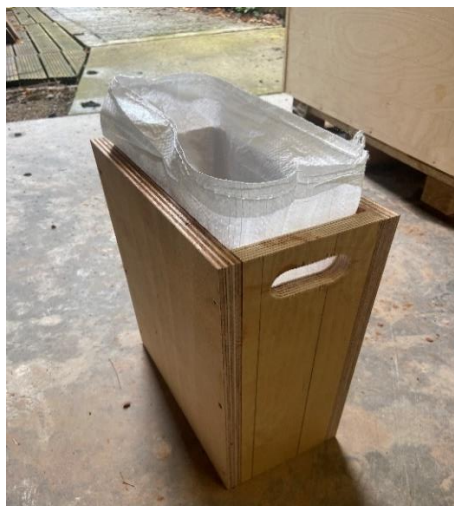
Fig. A. 1 Earthbag block mould
